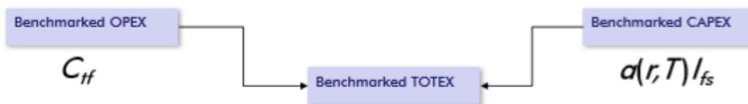
Figure 5.34 – Benchmarked TOTEX = OPEX + CAPEX 332
